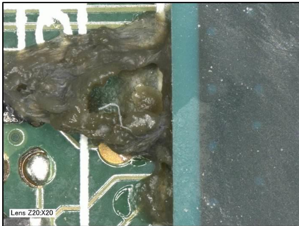
Figure 8-2: “Goop” With Whisker (courtesy of 3M)
