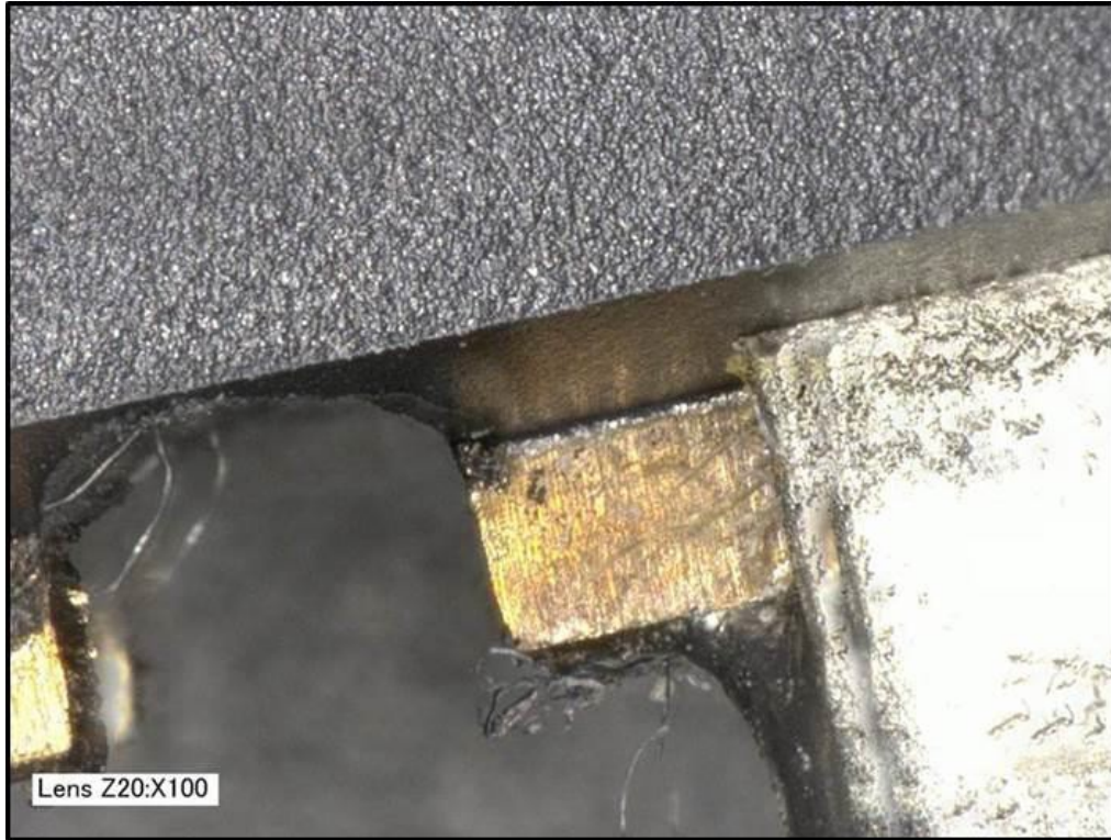
Figure 8-3: Metallic Whiskers (courtesy 3M)
