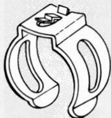
Retainer on tube clip has a self-retaining catch design.
