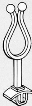
Purse-lock clips are interlocked to secure the wire bundle. Post clip tip snaps into a panel hole.
