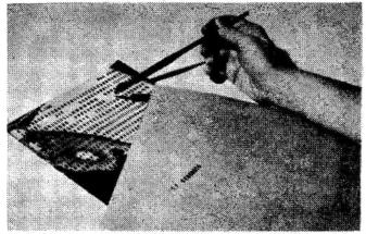
Planotype adhesive plastic letters are available in many colors and sizes. They are abrasion-resistant and recommended for front-panel use. Using a sharp-pointed instrument, lift the letters off the aluminum backing sheet and arrange them in word groups on the layout sheet. Complete word groups are lifted with transfer sheet.
