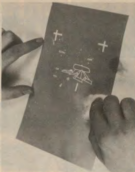
Three steps in making a Scotchcal panel (clockwise from top, left): 1. developing the negative; 2. developing the Scotchcal panel; 3. coating the finished panel with clear lacquer.
