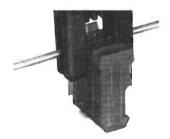
Lower MRT tool onto the connector with the guide rails over the wire.
