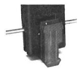
Firmly tap the tool until it bottoms out on the top of the connector. Repeat steps until connector is wired.
