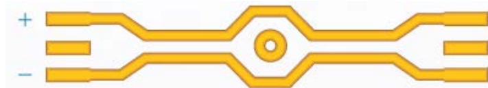
Fig. 4.17 Differential pair detouring of obstacles
