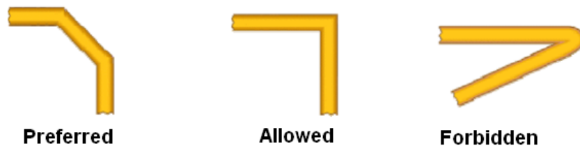
Fig. 8.8 Routing geometries and acid traps
