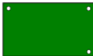
Fig. 7.1 Location of tooling pins
