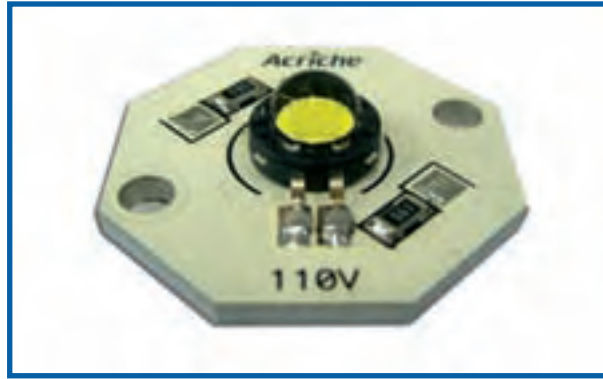
Figure 5. The Acriche LED modules from Seoul Semiconductor can be operated directly from the AC mains without a transformer. This is a 2-watt single-LED module. The manufacturer plans to boost the light yield from the current 48 lumen/W to 80 lumen/W in Q4 2007 and 120 lumen/W in 2008.
