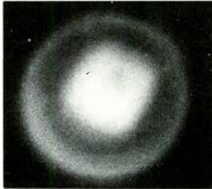
Fig. 6. Beam cross-section of a Stanley H1K with slightly misaligned chip.
