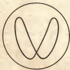
Fig. 3.7. Lissajous pattern created by feeding the scanning amplifiers with frequencies in the ratio 2 to 1
