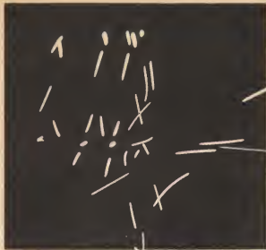
Fig. 3.6. The display produced by feeding different waveforms to the two deflection circuits. The higher frequency grid pulse produces the broken line effect
