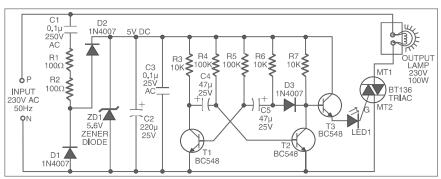
capacitors C1, C2, and C3, diodes D1 and D2, and zener ZD1 are used to develop a fairly steady 5V DC supply voltage that provides the required current to operate the multivibrator circuit and trigger triac BT136 via LED1.
