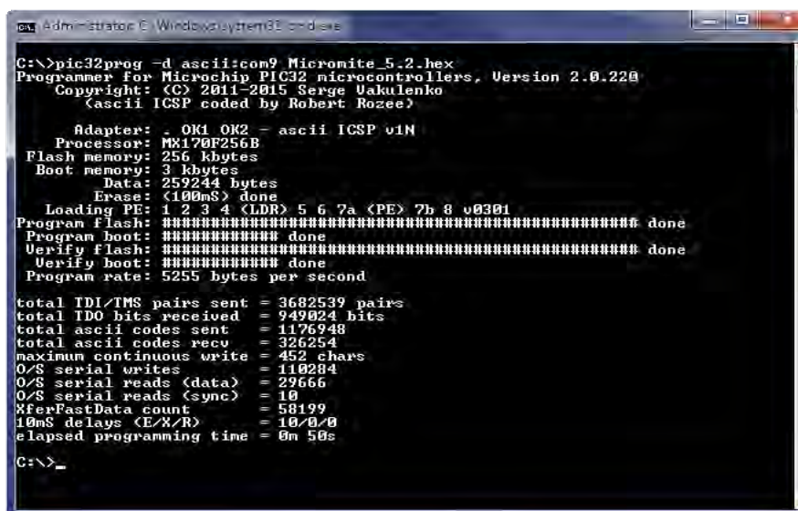
Fig.4: This screenshot shows the complete operation of pic32prog . It uploads the hex file to the Microbridge , which programs it into the PIC32 and subsequently reads back the programmed data to verify that the programming operation completed correctly.
