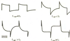
Fig. 5. Effect of the all pass filter on an ideal square wave of frequency f_1 .
