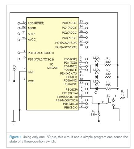
Atmel's (www.atmel.com) ATmega8 microcontroller (**Reference 1** and **Figure 1**). Listing 1, which is available at the Web version of this Design Idea at www.edn.com/080221di1, is a simple program for the circuit.
