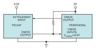
Figure 6 A pullup resistor on an open-drain output generates a 5V signal.
