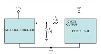
Figure 2 A resistive divider brings a 5V signal in range for a 3.3V input.
