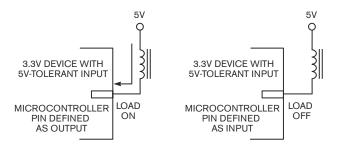
Figure 7 This circuit configuration drives low-impedance loads.
