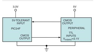
Figure 5 This simple interface works with 5V devices that have CMOS inputs.
