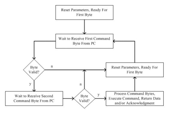
In the event custom firmware is required for a project, it is highly recommended the firmware is written and debugged separate of the PC software. This can be accomplished using a terminal program to emulate what is required of the PC during firmware development. This allows a separation of issues, and it can keep the debug time minimal.
