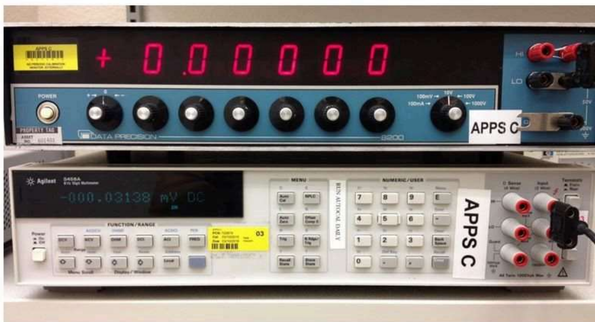
Figure 1: A low-noise voltage source and precision multimeter are two great analog debugging tools
