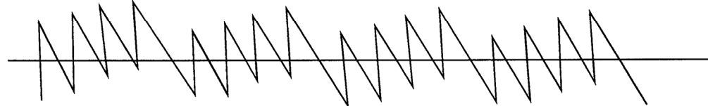
Figure 6.97: Idling Patterns for First-Order Sigma-Delta Modulator (Integrator Output)
