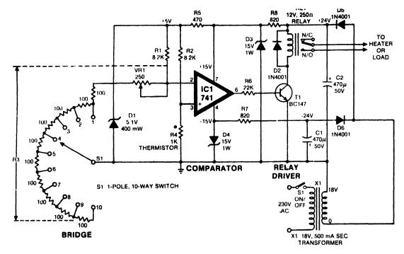
op-amp IC 741 and a 1k thermistor as the temperature sensor. It is based on the principle of wheatstone bridge. The ratio arms R1 and R2 of the bridge are kept fixed (say unity). The voltage across the thermistor, i.e. across the arm R4, is compared with the voltage across the variable arm R3 which is kept fixed for a particular temperature (using the op-amp).
