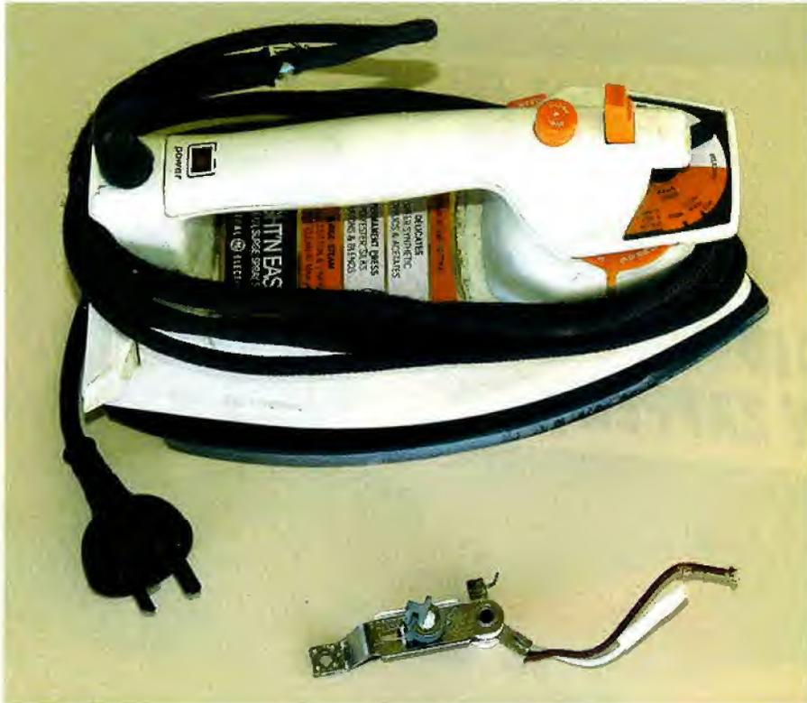
Every discarded electric iron has a thermostat mounted inside. These snap-action thermostats can be used to switch at temperatures from about 60-200°C.
