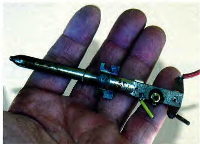
Electric frypan thermostats use a stainless steel probe that can be inserted through the wall of a pipe or into liquids. They can be adjusted to trip at temperatures from about 40-200°C.
