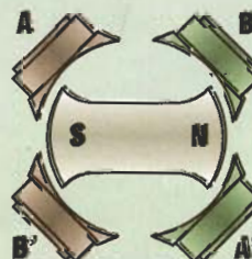
Step 7: Phase A: (-)ON Phase B: ON
