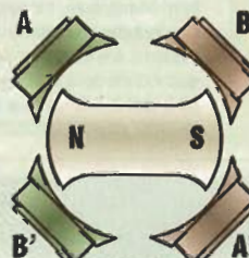
Step 3: Phase A: ON Phase B: (-)ON
