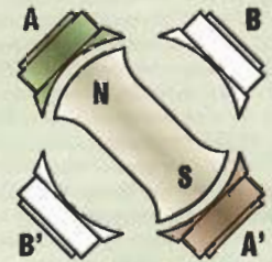
Step 2: Phase A: ON Phase B: OFF
