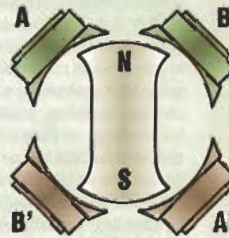
Step 1: Phase A: ON Phase B: ON
