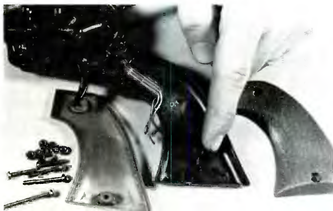
Photograph of the Coleco surplus plastic pistol modified by the author for use as a transmitter.
