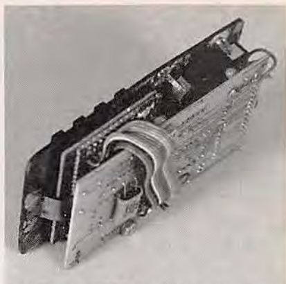
FIG. 10—THE PROTOTYPE TRANSMITTER is housed in a plastic case with a single-sided, copper-clad PC-board blank machined as its top panel.
