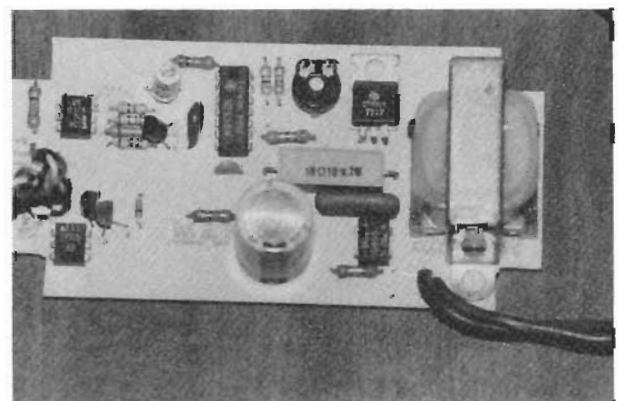
FIG. 8—THE CIRCUIT BOARD completely wired, ready for installation in the box.
