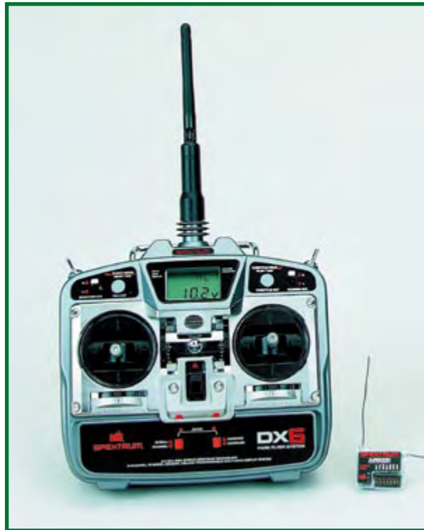
Figure 2. DX6 2.4 GHz model aircraft transmitter with receivers for six servo functions (Source: Graupner [6]).
