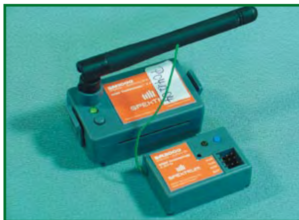
Figure 3. Transmit RF module and receiver for remote control of model cars (Photo: author).
