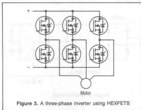
Figure 3. A three-phase inverter using HEXFETs
