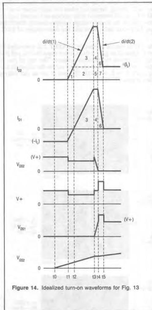
Figure 14. Idealized turn-on waveforms for Fig. 13
