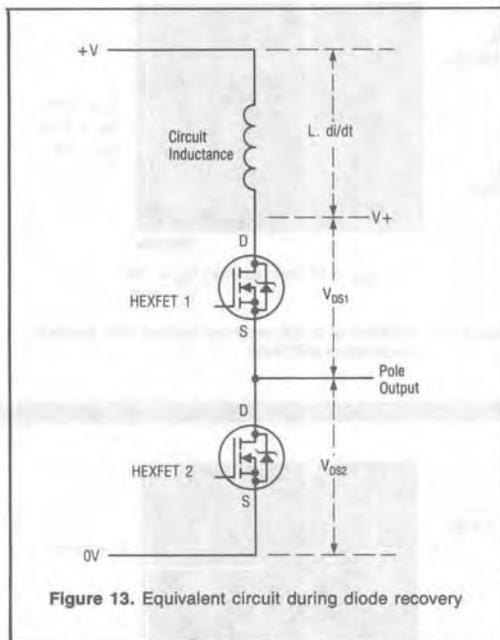
Figure 13. Equivalent circuit during diode recovery
