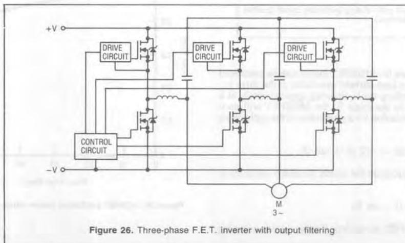
Figure 26. Three-phase F.E.T. inverter with output filtering
