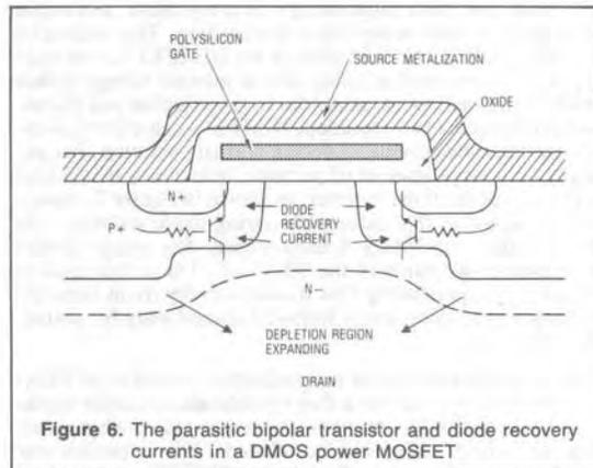
Figure 6. The parasitic bipolar transistor and diode recovery currents in a DMOS power MOSFET
