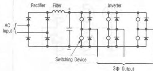
Figure 1. Inverter circuit
