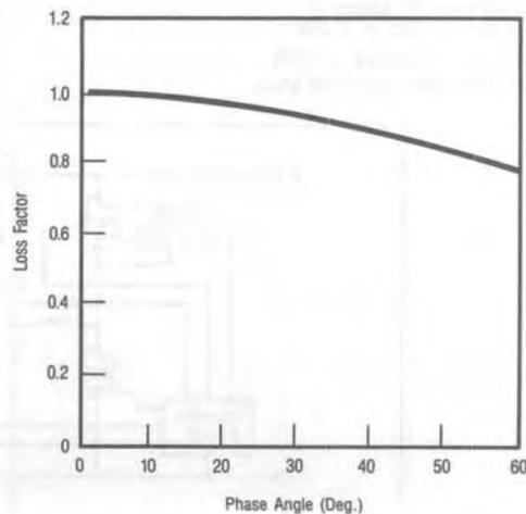
Figure 24. MOSFET conduction losses versus phase angle
