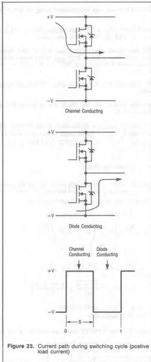
Figure 23. Current path during switching cycle (positive load current)
