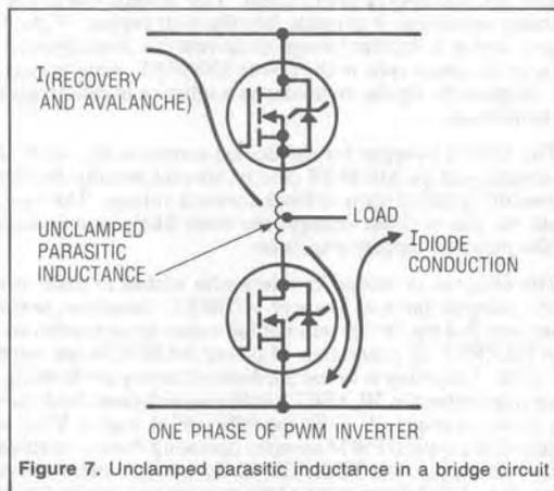
Figure 7. Unclamped parasitic inductance in a bridge circuit
