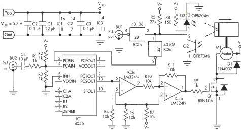
Used to maintain motor M1's speed and phase, this circuit requires fewer parts than a conventional solution and eliminates the loop filter entirely.
