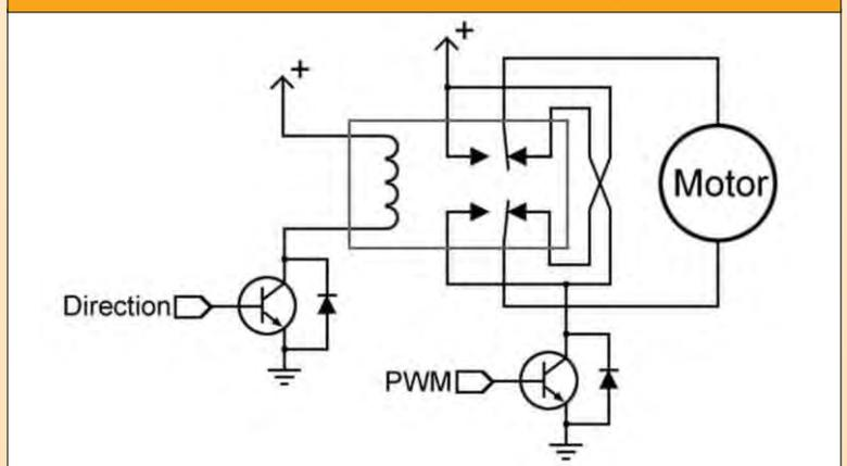
over again. The amount of time that you have the motor on versus off determines the average speed of the motor.
