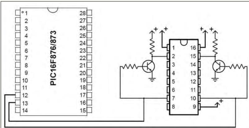
Figure 8. Controlling a motor using Locked Anti-Phase PWM.
