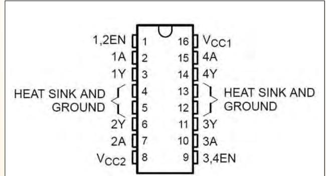
Figure 5. Pinout for the L293D.
