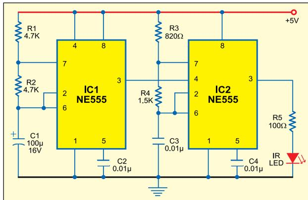
Fig. 1: Infrared transmitter
