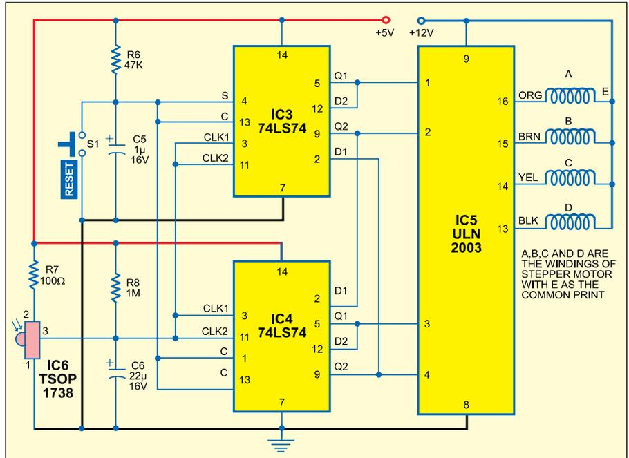
Fig. 2: Infrared receiver and stepper motor driver circuit
