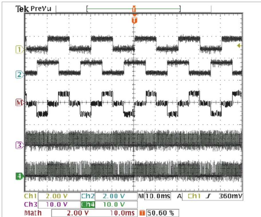
Figure 2 Waveforms from the circuit in Figure 1 include the A\_Step input (Channel 1), B\_Step input (Channel 2), outputs OUTR+ (Channel 3) and OUTR- (Channel 4), and the signal that arrives at the motor's windings (OUTR+ minus OUTR-, middle trace), which the oscilloscope's math function computes.
