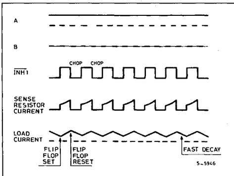
Figure 19 : The Chopper oscillator of multiple L297s are synchronized by connecting the SYNC Inputs together.
