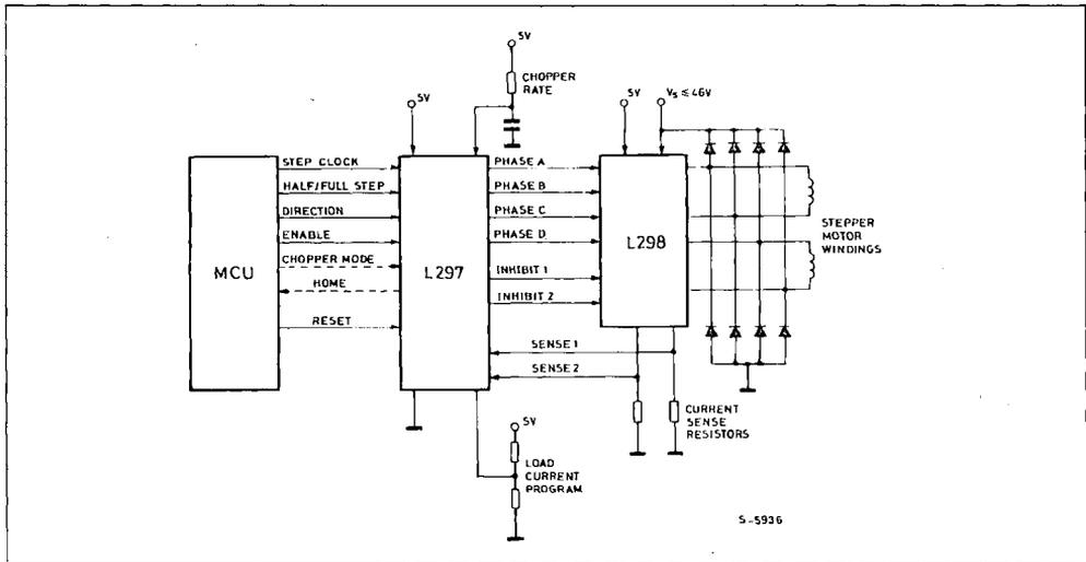
For bipolar motors with winding currents up to 2A the L297 should be used with the L298N ; for winding currents up to 1A the L293E is recommended (the L293 will also be useful if the chopper isn't needed). Higher currents are obtained with power transistors or darlingtontons and for unipolar motors a darlington array such as the ULN2075B is suggested. The block diagram, figure 1, shows a typical system.
