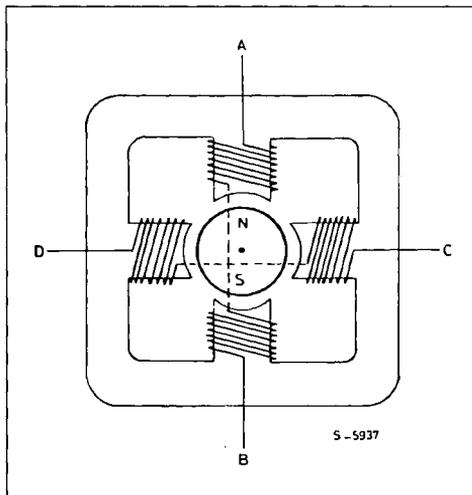
The first is to energize the windings in the sequence AB/CD/BA/DC (BA means that the winding AB is energized but in the opposite sense). This sequence is known as "one phase on" full step or wave drive
