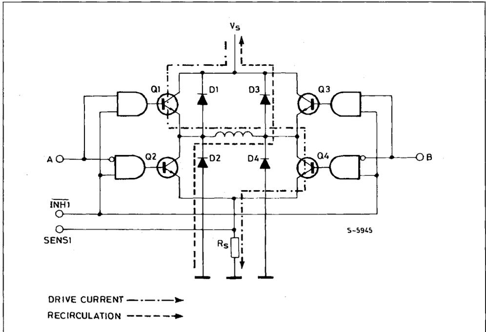
In this case when the voltage across  $R_S$  reaches  $V_{REF}$  the chopper flip flop is reset and INH1 activated (brought low). INH1, remember, turns off all four transistors therefore the current recirculates from ground, through D2, the winding and D3 to  $V_S$ . Discharged across the supply, which can be up to 46V, the current decays very rapidly (figure 18).
