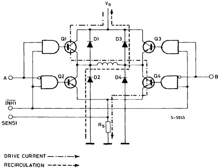
The L297 provides load current control in the form of two PWM choppers, one for each phase of a bipolar motor or one for each pair of windings for a unipolar motor. (In a unipolar motor the A and B windings are never energized together so they can share a chopper; the same applies to C and D).
