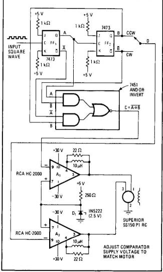
**Stepping a synchronous motor.** Logic circuit plus high-power comparators step two-phase synchronous motor in clockwise or counterclockwise direction. Frequency of input square wave determines motor stepping speed. Two-bit counter formed by flip-flop pair and AND-OR-INVERT circuit produce four logic outputs (A, B, C, and D) that control motor. Each comparator output supplies one motor coil.
