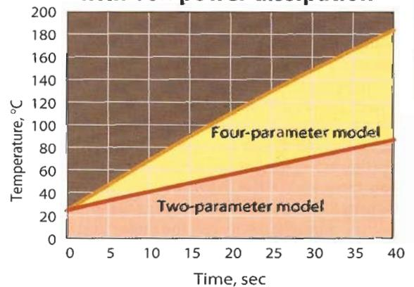
The four-parameter model predicts the winding reaches its rated 130°C value in only 25 sec while the two-parameter model predicts winding temperature should only be 62°C at this point. Experiments confirmed the prediction of the four-parameter model.
