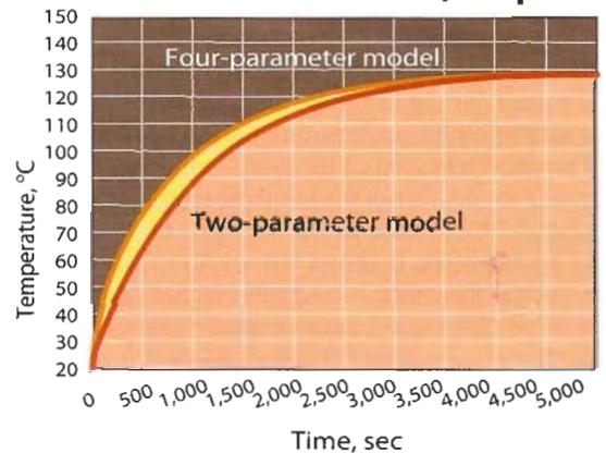
The four-parameter thermal model predicts winding temperature will rise more quickly than does the standard two-parameter model for a 60-mm servomotor, with  $1\times$  continuous power dissipation.
