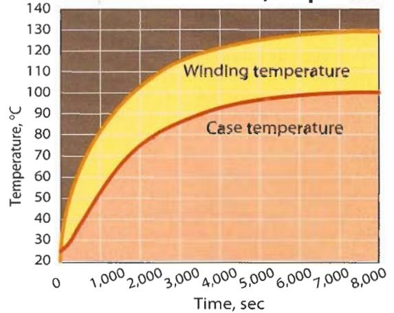
Measured temperatures on the windings and case of a 60-mm servomotor show where the temperatures stabilize with  $1\times$  constant power dissipation.
