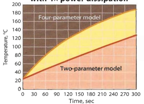
The four-parameter model predicts the winding heats to its rated 130°C value in 140 sec. The two-parameter model says the winding should be less than 80°C at this point. Experimental measurements confirmed the four-parameter prediction.
