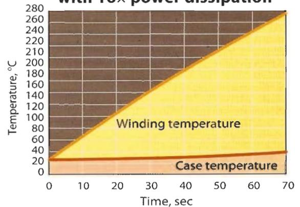
The four-parameter model predicts the winding temperature will rise rapidly to its 130°C rated value. During this same time period the case temperature hardly changes. The two-parameter model predicts the winding temperature (graph not shown) will be less than its 130°C rated value at 70 sec. Actual measurements show the winding is at or above 280°C at this point and in the process of burning up.
