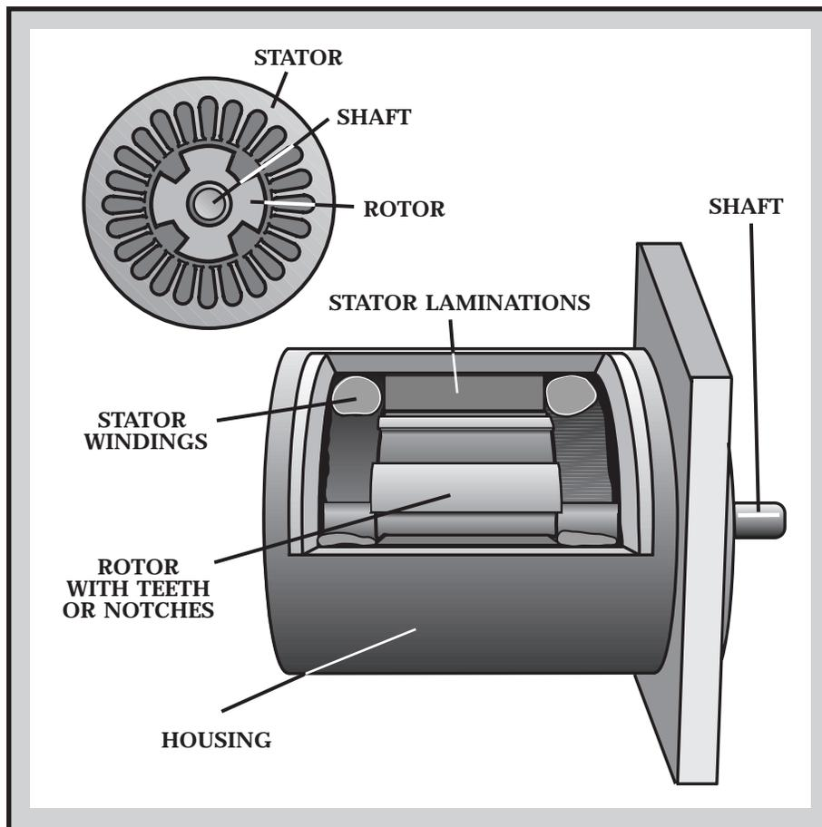
Fig. 4 - CUTAWAY OF AC SYNCHRONOUS MOTOR
