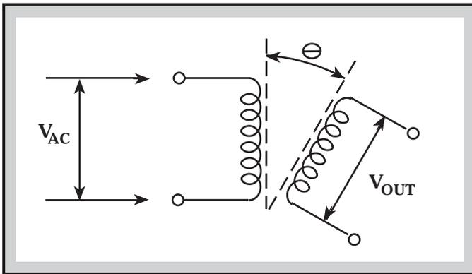
Fig. 25 - RESOLVER: A ROTATING TRANSFORMER
