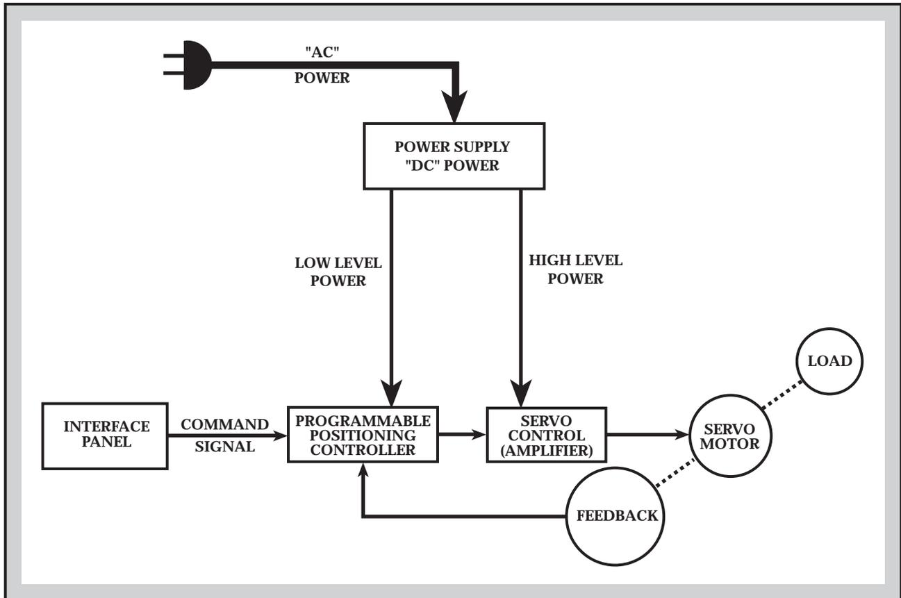
*Fig. 13 - THE CONCEPT OF A SERVO SYSTEM*
