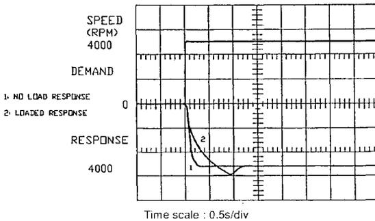
**Figure 10 :** The Effect Upon the Dynamic Response of the Analogue Velocity Servo System, When the Gain of the Proportional Term in the PID Controller is Varied.
