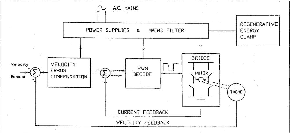
**Figure 2 : Schematic Diagram of Brush D.C.P.M. Motor Drive.**
