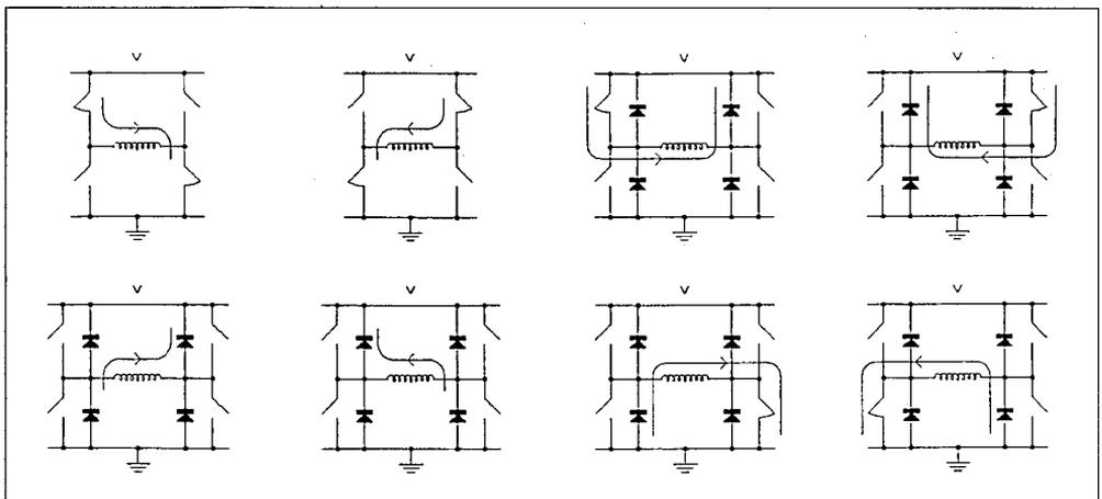
Figure 6 : 6kVA MOSFET Switch Configurations Using ISOFETs and FREDs.
