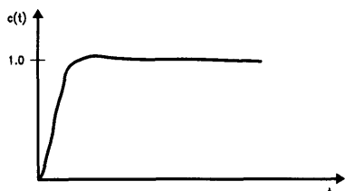
FIGURE 20. Unit Step Response of a Critically Damped System
