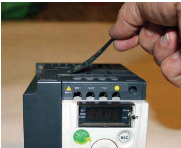
Figure 1 Remove the vent covers for Type B or C mounting when IP20 protection is adequate, but leave them on the housing in Type A mounting.
