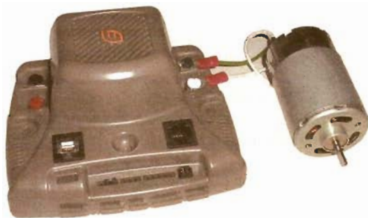
4. Luminary Micro's RDK BDC BLDC reference kit is representative of motor control kits that come with a motor. The 32-bit Cortex-M3 core is available with communication interfaces such as Ethernet and CAN.
