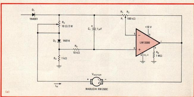
**Speedy solution.** One-chip power op-amp circuit (a) makes simple, low-cost speed control for small dc motors. Circuit affords excellent common-mode rejection. Controller's rpm-vs-load performance (b) is superior to that of circuits utilizing a constant-voltage drive.
