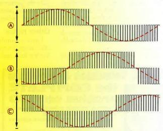
the amplitude of the drive voltage must be reduced as the frequency is lowered.
