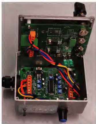
Inside the Motor Speed Controller – full construction details will be presented next month but will be slightly different from this prototype. The links on the motor PCB have been set up for high-side operation.
