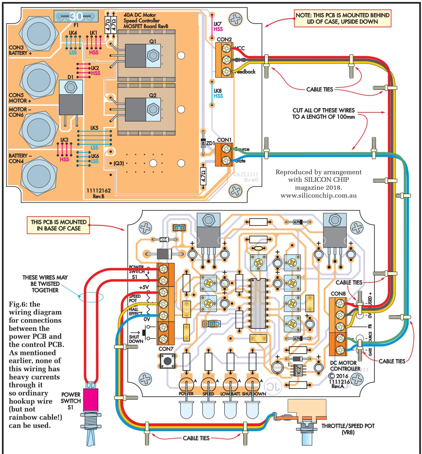
Fig.6: the wiring diagram for connections between the power PCB and the control PCB. As mentioned earlier, none of this wiring has heavy currents through it so ordinary hookup wire (but not rainbow cable!) can be used.
