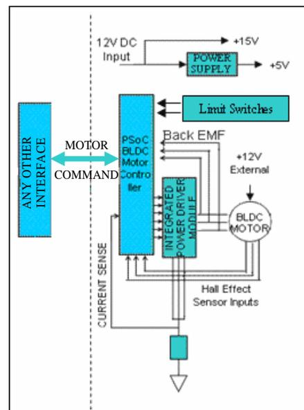
Figure 17. PSoC Automotive BLDC Interfacing to Other Systems
