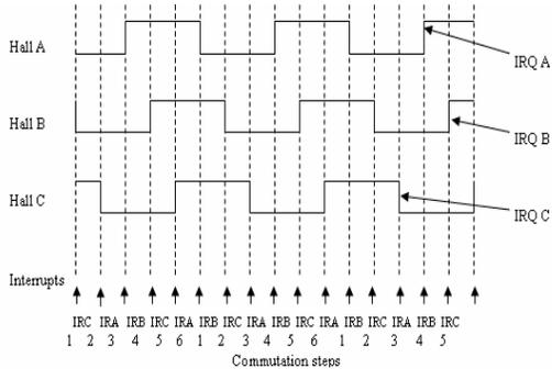
Figure 9. Output of Hall-Effect Sensors
