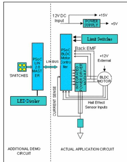
Figure 12. PSoC Automotive BLDC Block Diagram
