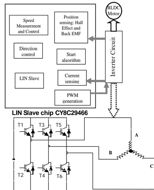
Figure 6. Main Blocks of BLDC Motor Control
