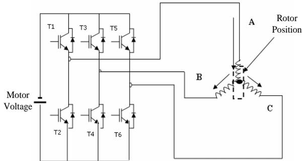
Figure 10. Alignment Phase Triple Half Bridge
