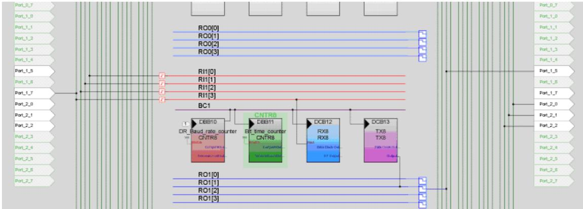
Figure 14. PSoc Designer Digital Blocks used for LIN Slave Data Reception Configuration
