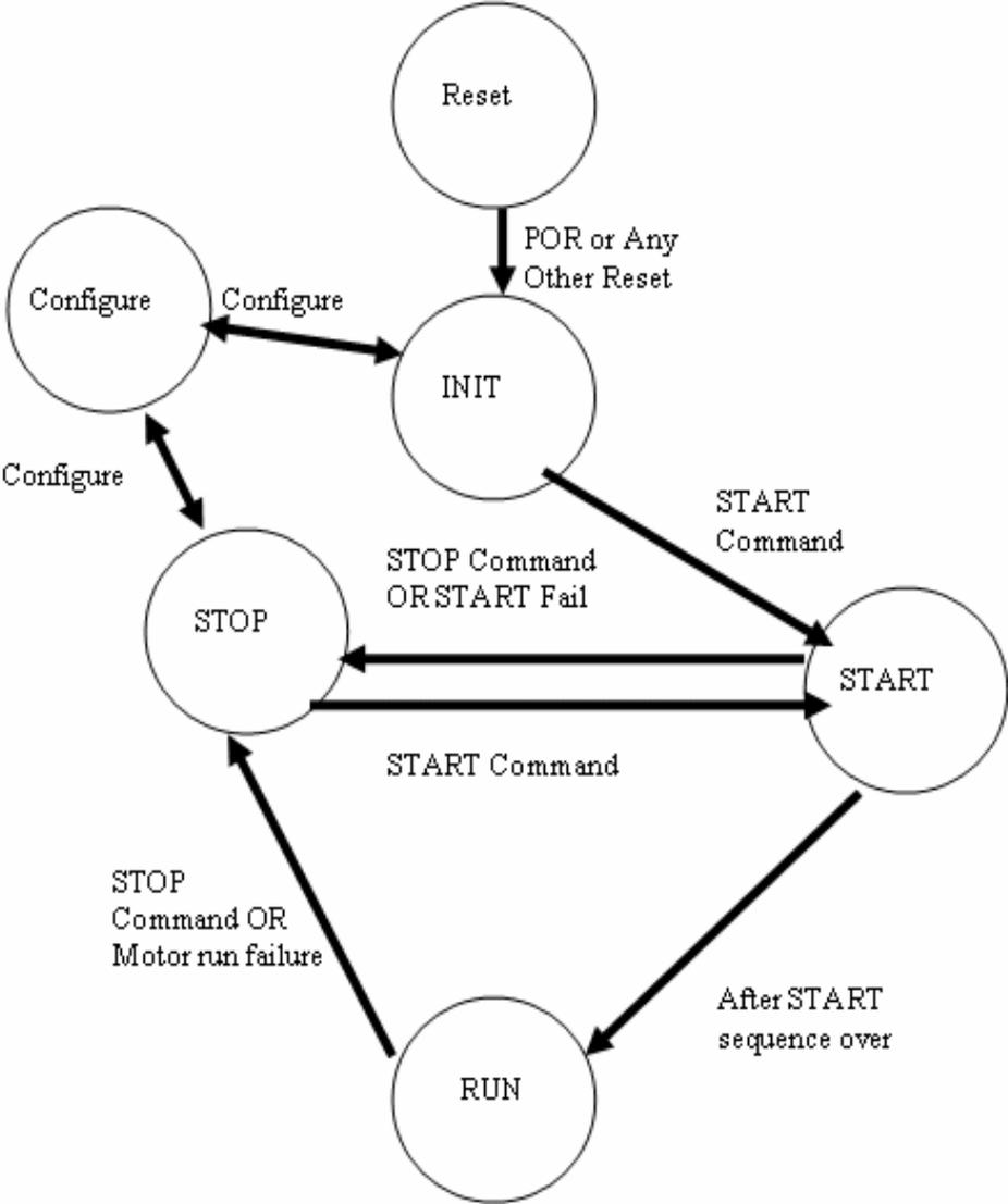
Figure 20. Motor Control State Machine
