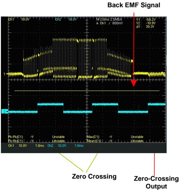
Figure 8. Back EMF Zero-Crossing Detection, Zero-Crossing Signals
