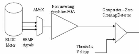
**Figure 7. Zero-Crossing Detection (Sensor-Less Mode)**
