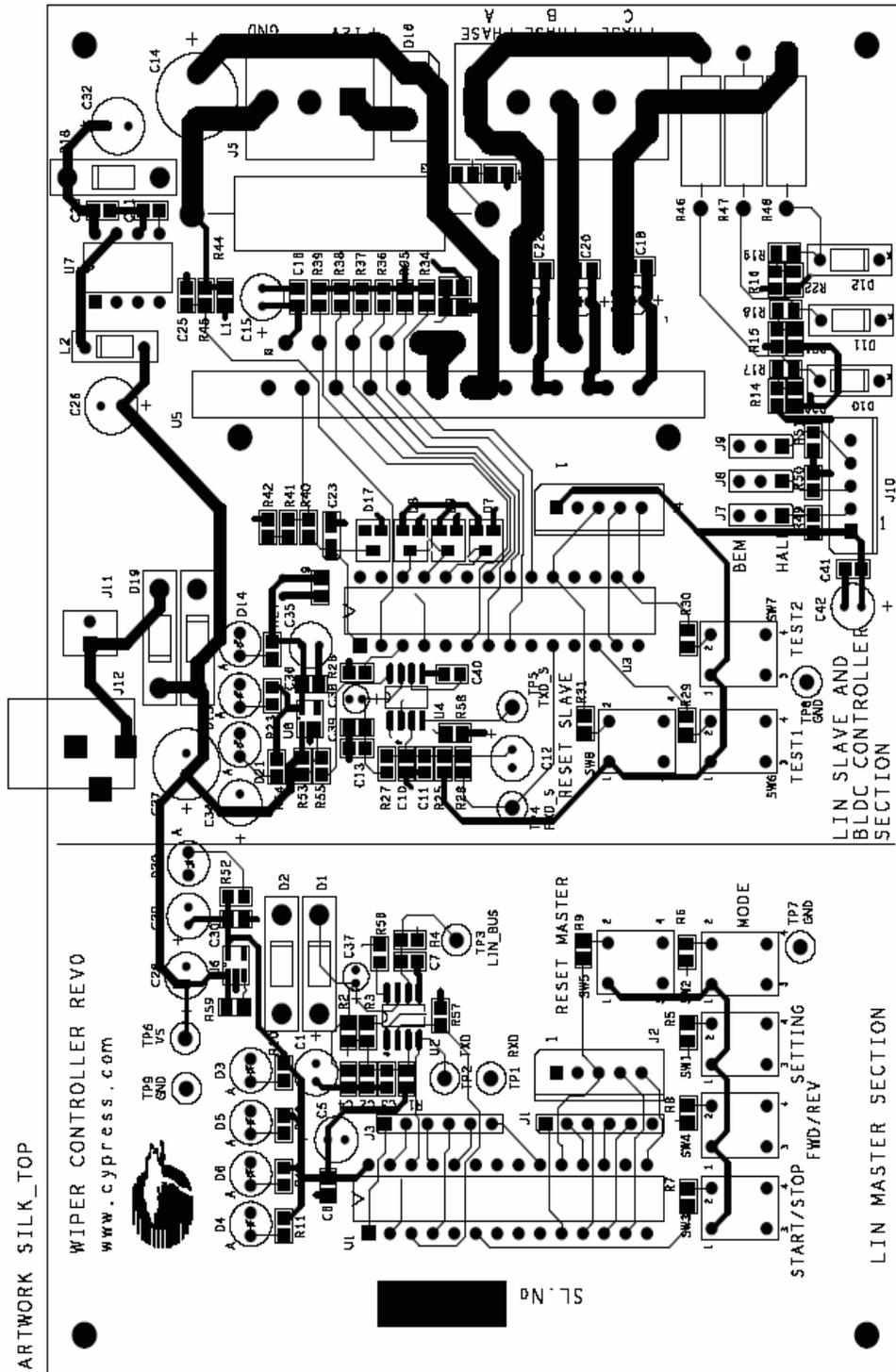
Figure 28. BLDC Motor Control Board Component and Track Layout
