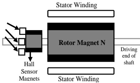
Figure 1. BLDC Motor Transverse Section
