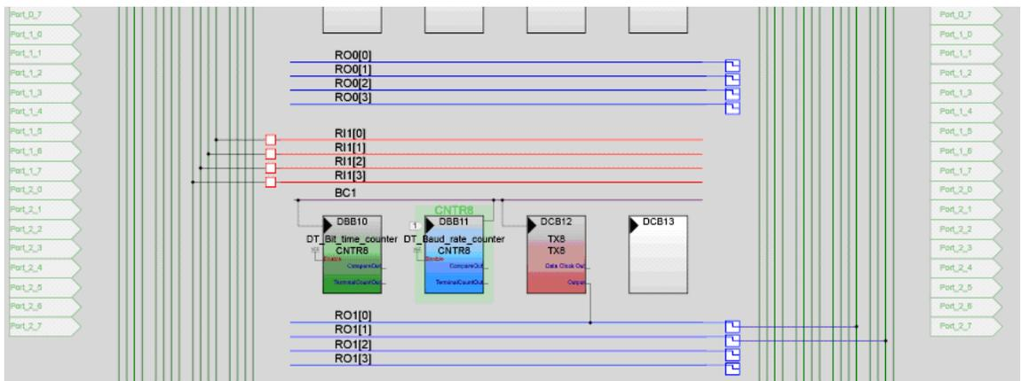
Figure 15. PSoc Designer Digital Blocks used for LIN Master Data Reception Configuration
