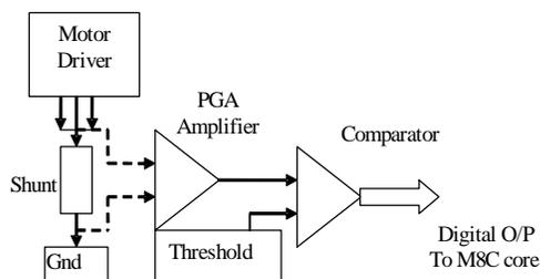
Figure 11. Current Measurement
