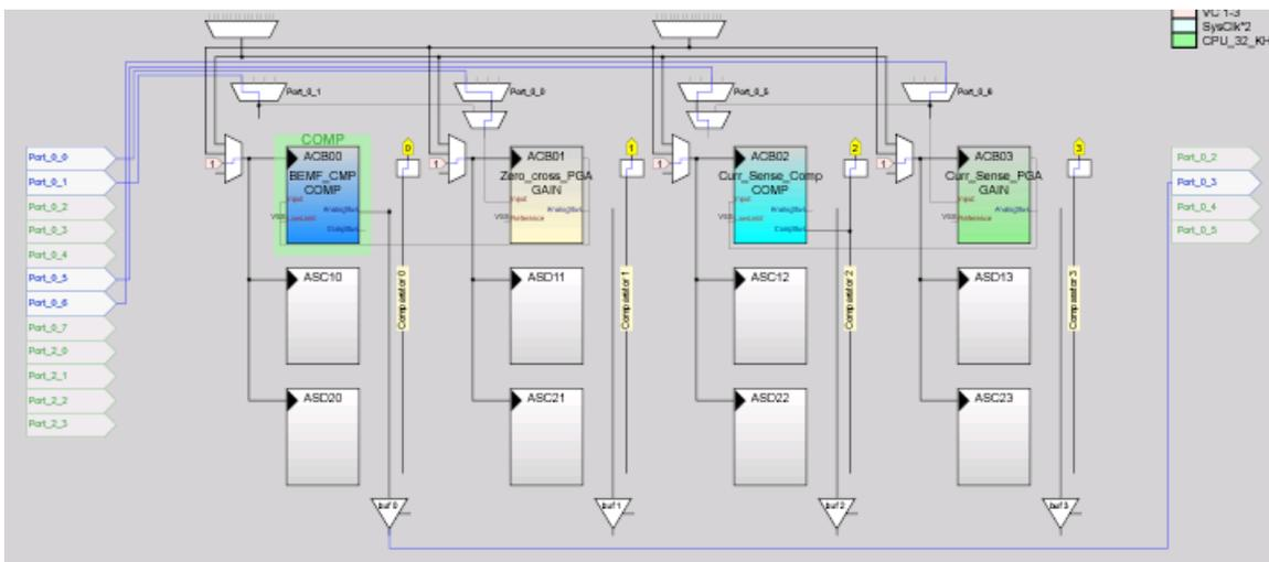
Figure 16. PSoc Designer Analog Blocks used for LIN Slave and BLDC Motor Controller
