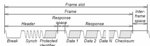
Figure 2. Structure of a LIN Frame
