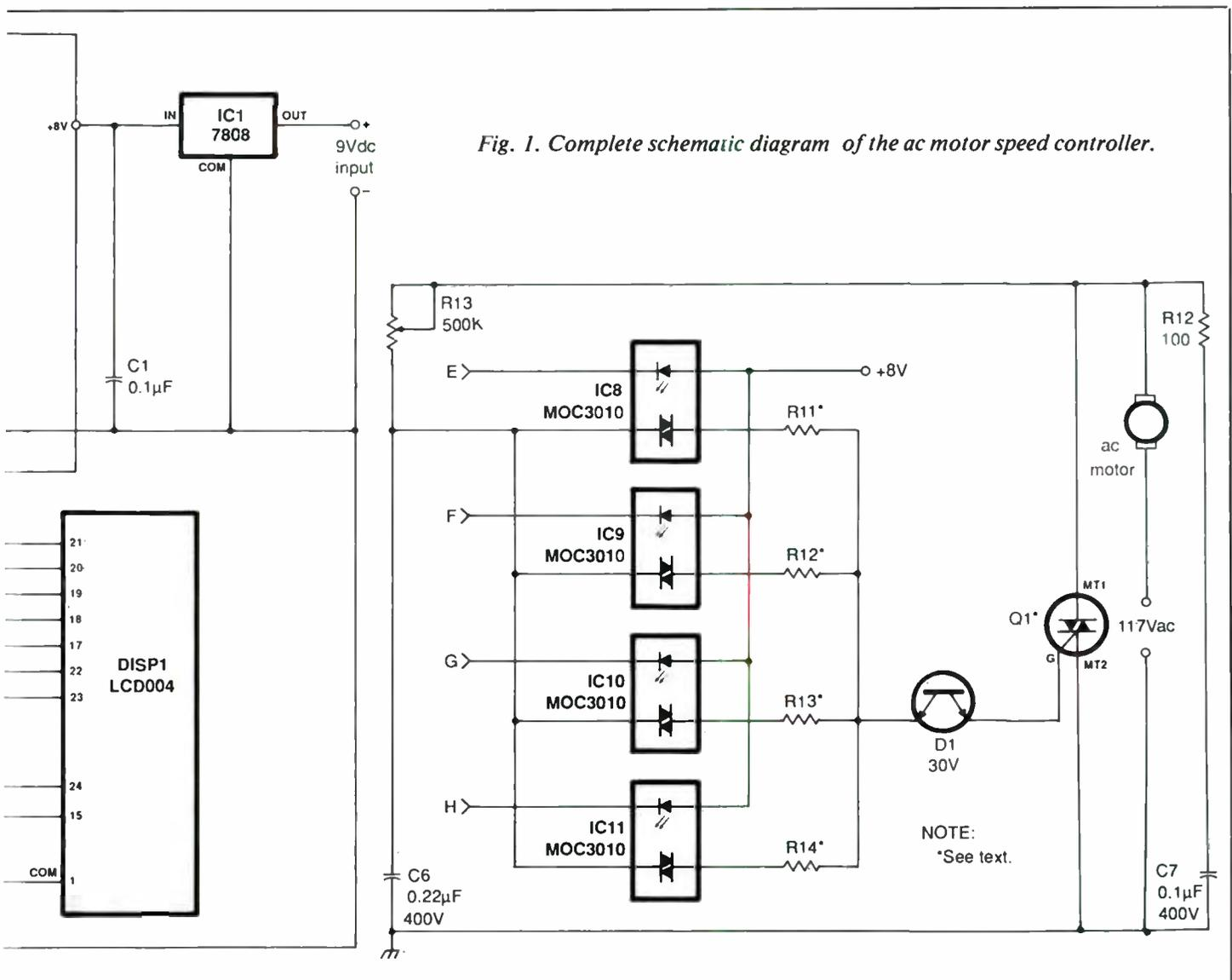
Fig. 1. Complete schematic diagram of the ac motor speed controller.
