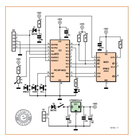
Figure 1. The transmitter circuit.
