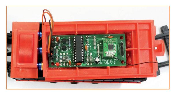
grammer. Free software downloads for this project from the Elektor site include the ready-assembled firmware and Pascal source file. Firmware for this project can be compiled using versions 5.60 or 6.01 of Pascal Pro from MikroElektronika [6]. The fully functional compiler is free to use for programs less than 2 KB in size. The microcontroller connector K2 hooks up to a Microchip PICKit3 programmer [7] for in-circuit programming.
