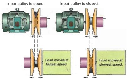
Some belt systems are mechanically linked so that as one pulley is open or closed, the opposing pulley is changed as well — to regulate speed.
