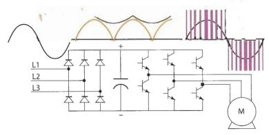
By separating torqueproducing current from that for flux, vector drives can produce full torque down to zero rpm. Note that horsepower remains constant beyond base speed — impossible with certain mechanical systems.
