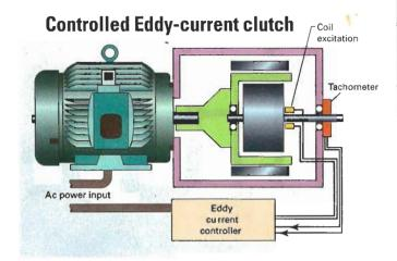
In a system using an Eddy-current clutch for speed control, the motor is started while the clutch is disabled. After the motor has reached its speed, a controller engages the clutch by allowing current to flow to it.
