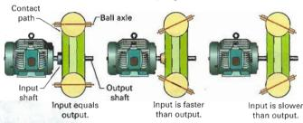
Or, as shown here, drive balls mounted on tiltable shafts press upon cone faces. By moving a lead screw, the balls tilt the shafts to increase or decrease the overall speed ratio.
