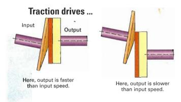
In traction drives, two rotors mesh at varying angles. Changing the contact adjusts load speed.
