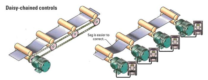
Instead of using one 20-hp motor with mechanical links to synchronize motion, four 5-hp drives with motors can be used instead. This eliminates the wear that can cause asynchronous motion.
