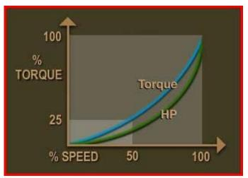
C Variable torque loads include most centrifugal and axial pumps, fans and blowers and many mixers and agitators.
