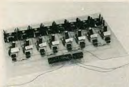
FIG. 6—CONNECTION to the AC controller is made through DIP header. Ribbon cable may be used instead of individual wires.
