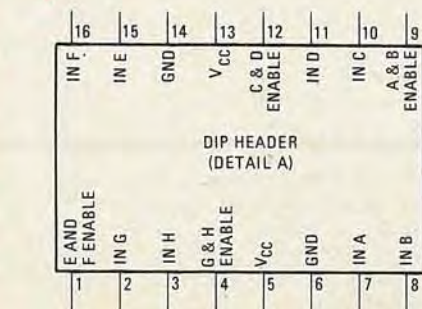
FIG. 5—ALL THREE LEADS of the outermost triacs are brought out to edge of board (see text). Detail "A" shows pinout of DIP header for connection to computer.
