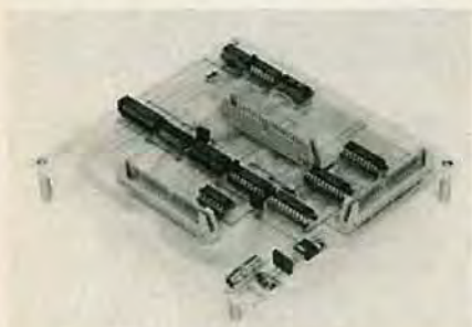
FIG. 13—USE THE TRS-80 INTERFACE as shown or, better, enclose it in a protective case for security.
