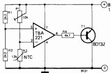
The NTC resistor forms one arm of a Wheatstone bridge (R1, R2, R3 and P1). The unbalance voltage from the bridge is applied to the differential input of the TBA 221 op-amp, which operates as a low-hysteresis voltage comparator. The op-amp quickly saturates in one direc-
