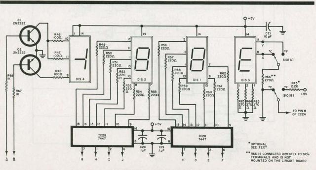
Fig. 4. Schematic of the display circuit.
