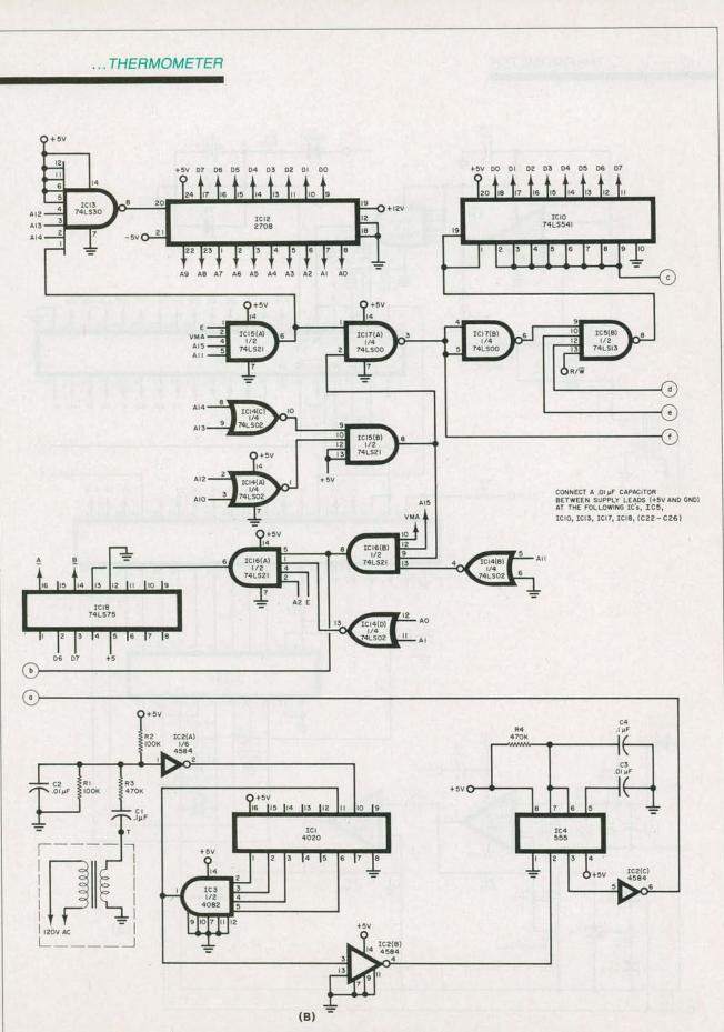
Fig. 3B. EPROM and logic circuits.
