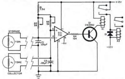
The Solar Controller is a temperature comparator that turns on a blower or pump when the air or fluid in the solar collector is at a sufficiently high temperature to justify a transfer to the storage medium. In the fan application, control is by the temperature difference between the attic and outside air (or between ceiling and floor of a large room).
